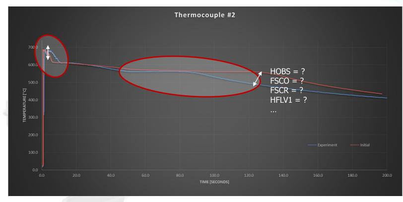
The goal of this study is to optimize numerical parameters to set in *FLOW-3D* to match both the <u>filling dynamic</u> and the <u>solidification behavior</u>.
