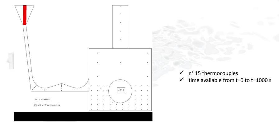
A gravity casting pouring, with well known data and a mold fully filled of thermocouples.
