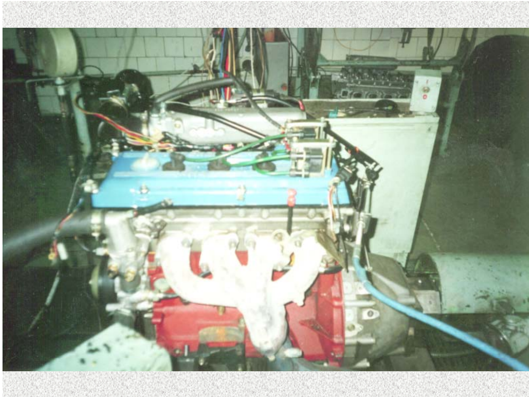
Figure 7. Experimental test stand for the AvtoVAZ car engine.
